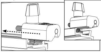
Align the threaded screw of the Micro-Adjuster with the accessory hole in the Clamp Block. Thread the Micro-Adjuster screw into the Clamp Block by rotating the Micro-Adjuster Thumb Wheel until the screw is roughly 3/4 of the way threaded into the Clamp Block.
